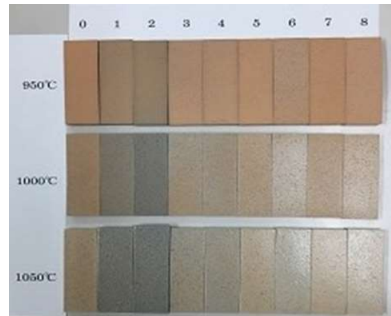
Fig. 3: Appearance of ceramic samples made in 950, 1000, and 1050 degrees Celsius
