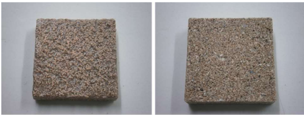
Fig. 5: Appearance of porcelain tiles (left) and water-permeable tiles (right) made from pretreated glass cullet
