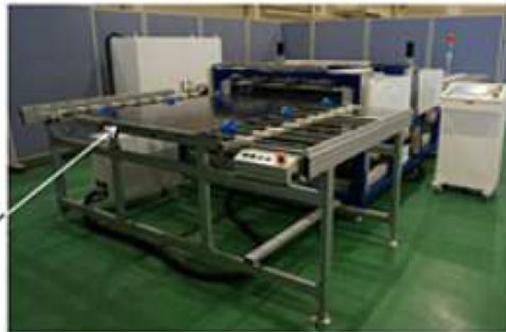
Glass separating equipment with a hot cutter
