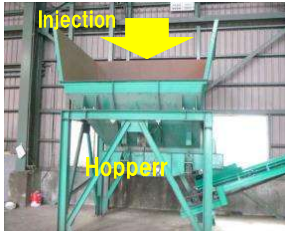
① Injection into hopper with a forklift for the PV panel waste which it crushed with a shredder
