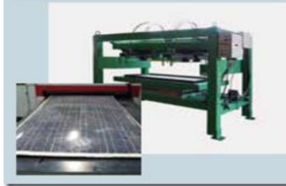
Removing Aluminum Frames
